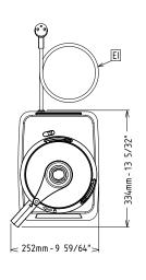
Electric Supply voltage: 220-240 V/1N ph/50 Hz Electrical power, max: 0.5 kW 0.5 kW **Total Watts:** Capacity: Performance (up to): Capacity: 3.6 litres Key Information: External dimensions, Width: 252 mm External dimensions, 334 mm Depth: External dimensions, Height: 476 mm **Shipping weight:** 18.2 kg Meat mincing capacity: 0 kg Mayonnaise preparation 0 kg capacity: Pastry preparation capacity: 0 kg
